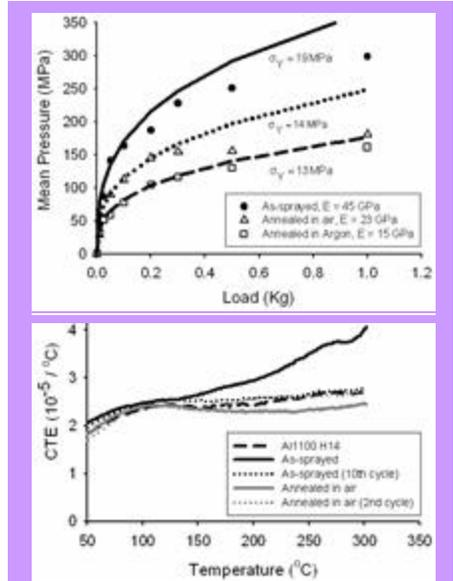
(top) Modulus and yield strength results from indentation, (bottom) CTE measurements.
