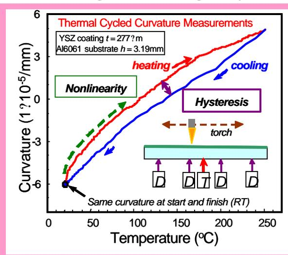
Measured temperature and curvature of YSZ coating/Al substrate during a thermal cycle test. During loading and unloading, the coating exhibits nonlinear and hysteretic stress-strain behavior. Curvature measurement system is shown at inset; thermal cycling tests are accomplished by heating the bi-layer with a torch and continuously recording backside displacement.
